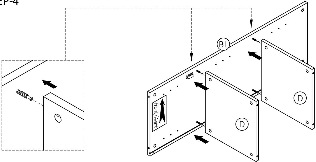
1. Align Cam Lock Pins with guide holes on parts (D) and attach parts (D) to Left Side (BL).
