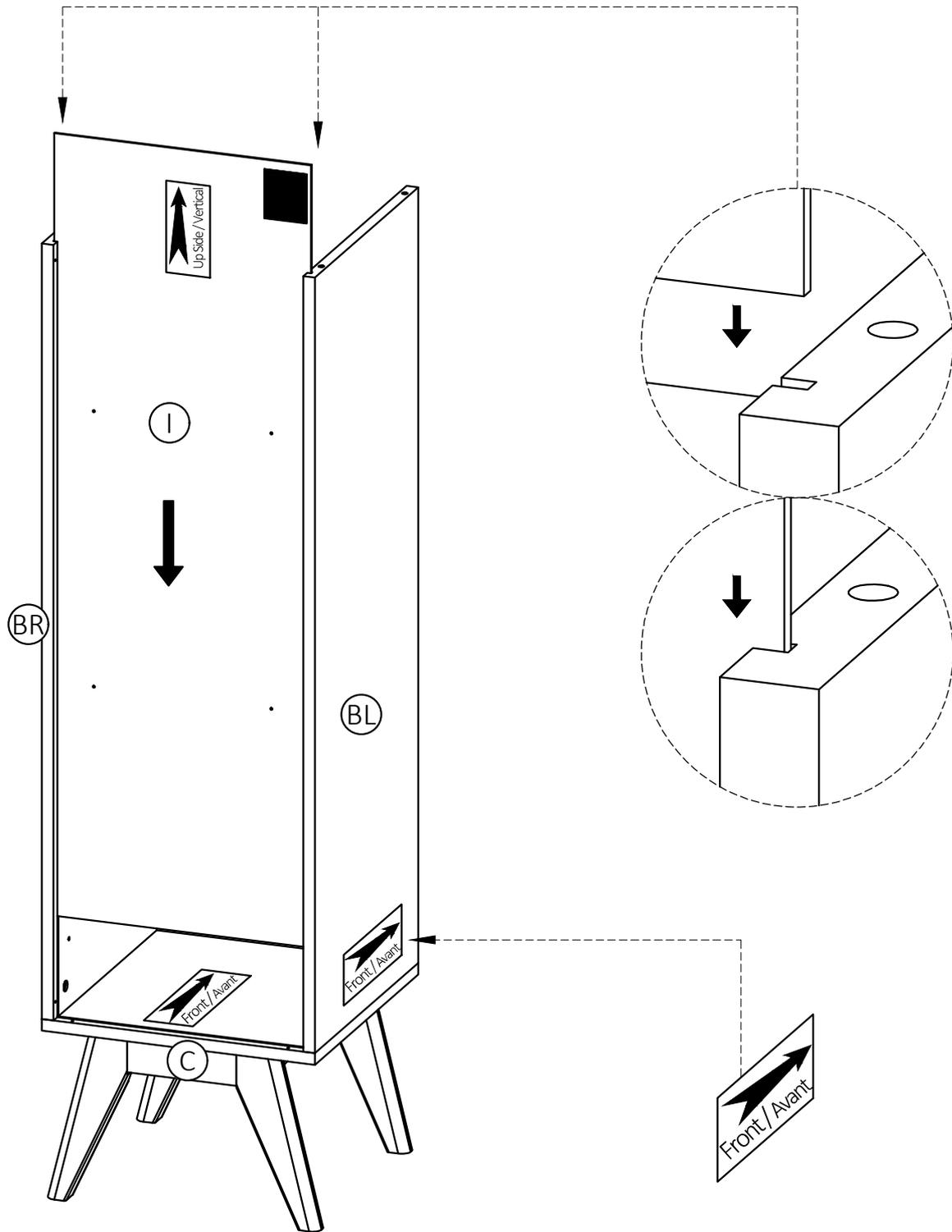
1. Slide Back Panel ① firmly into slots on Sides ②L, ②R and Bottom Shelf ③.
