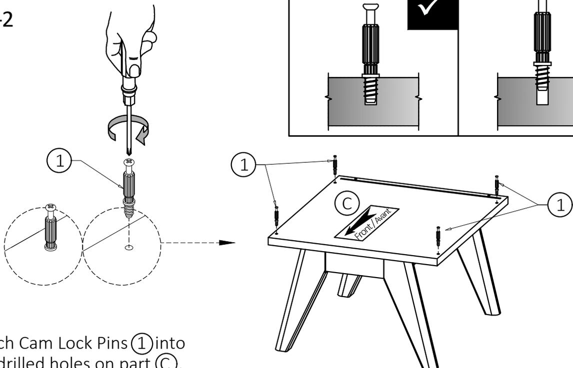
1. Attach Cam Lock Pins (1) into pre-drilled holes on part (C).
