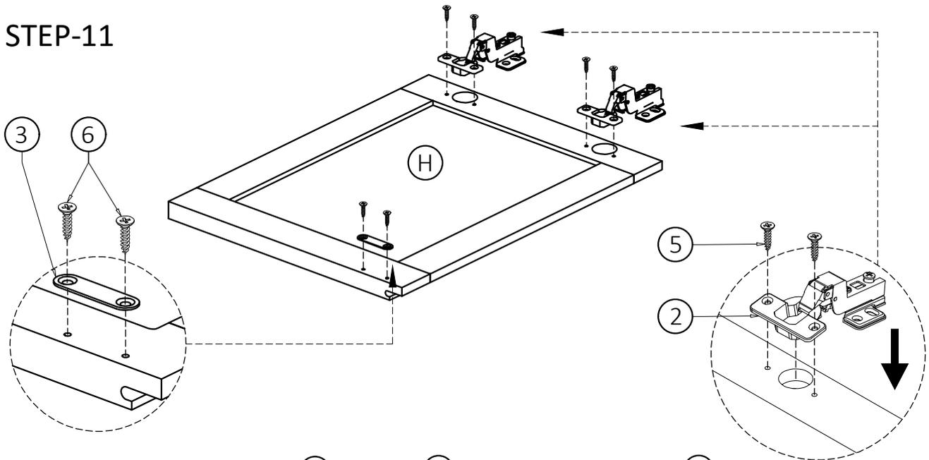
1. Attach Adjustable Hinges (2) to Door (H) using Phillips Screws (5) into pre-drilled holes on Door (H).
