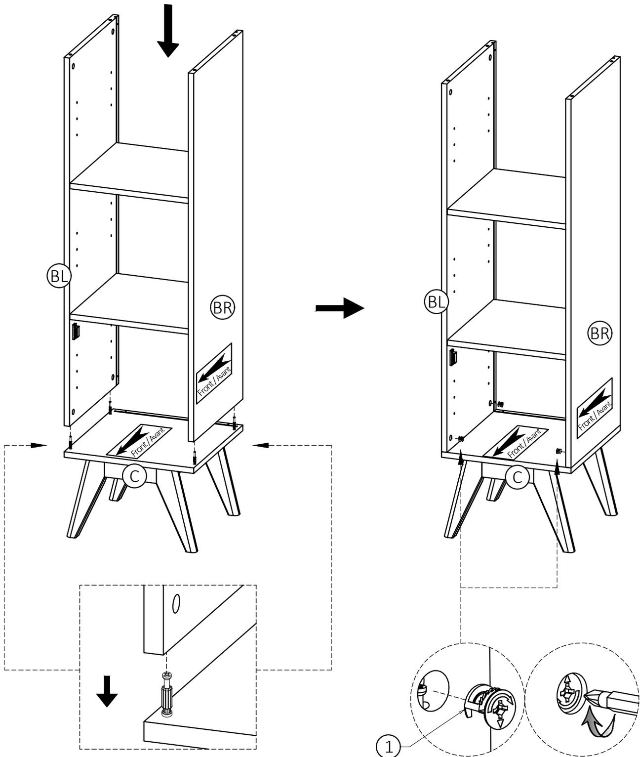
1. Align Cam Lock Pins with guide holes on parts (BL), (BR) and attach part (C) to parts (BL), (BR).
