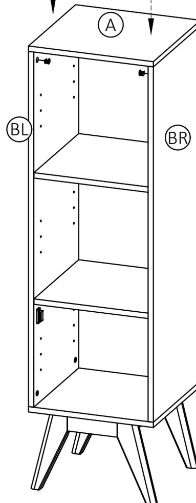
1. Align Cam Lock Pins with guide holes on parts (BL), (BR) and attach part (A) to Sides (BL), (BR).
