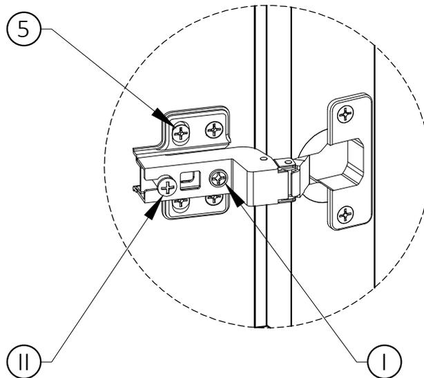
Tighten the Screw marked (II) to fasten hinge. The door may need to be adjusted so that all the spaces between the door and the unit sides are equal.
