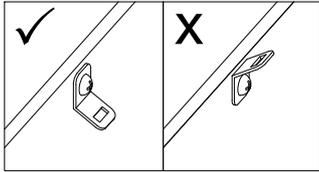
2. Determine where furniture is to be placed and mark location on the wall for mounting bracket screw hole approximately 2 inches **below** the bracket mounted to the furniture.
