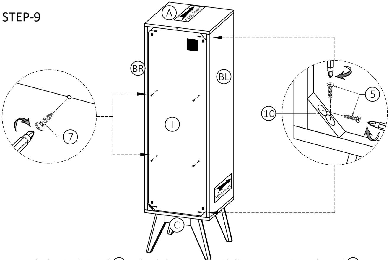
1. Attach the Back Panel (1) to back frame using Phillips Screws Round Head (7) through guide holes from Back Panels.
