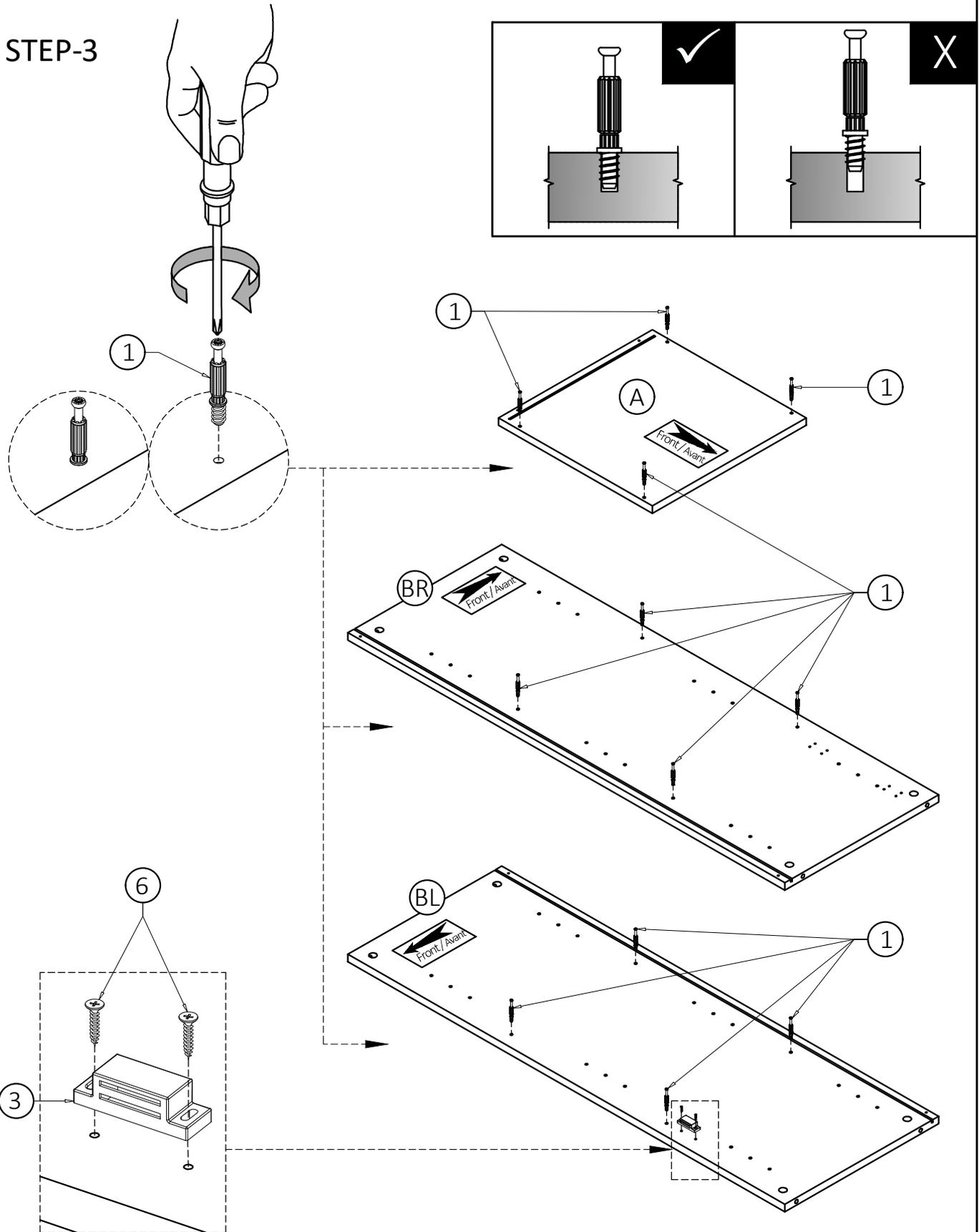
1. Attach Cam Lock Pins ① into pre-drilled holes on parts (A), (BL), (BR).
