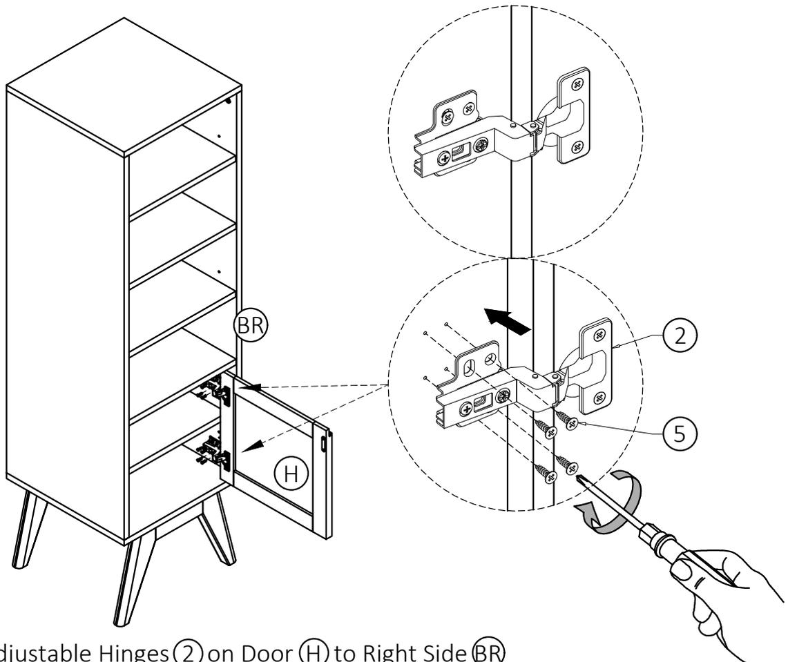
1. Attach Adjustable Hinges (2) on Door (H) to Right Side (BR) using Phillips Screws (5) into pre-drilled holes on Right Side (BR).
