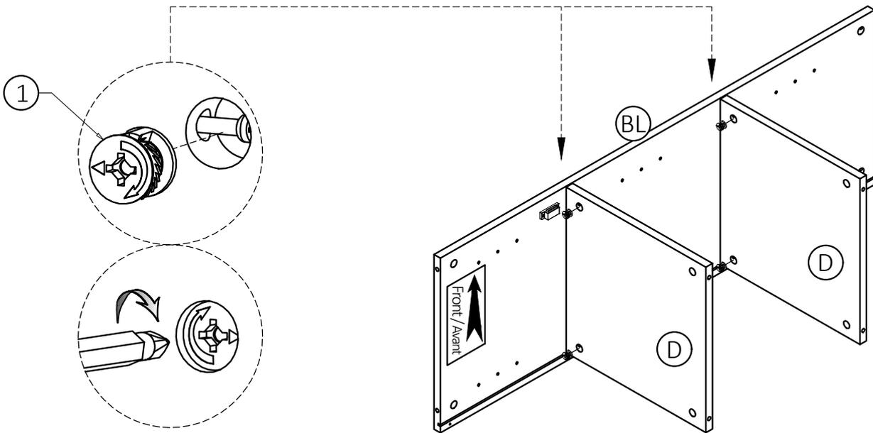
2. Insert two Cam Locks (1) into guide holes on each part (D).
