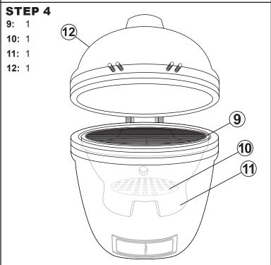
Ensuring the bottom vent faces the front, place Kamado Grill (12) in the stand. Insert Firebox (11), Charcoal Grate (10) and Cooking Grate (9) into the grill.
