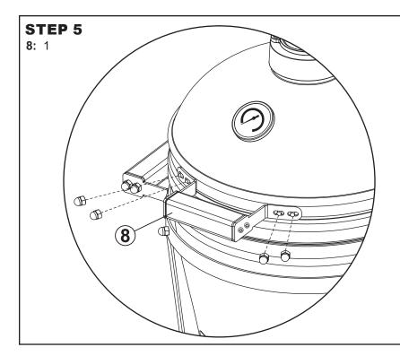
Remove the cap nuts from the threaded posts on the grill lid. Install Grill Handle (8) over the threaded posts and use the cap nuts to firmly secure it.
