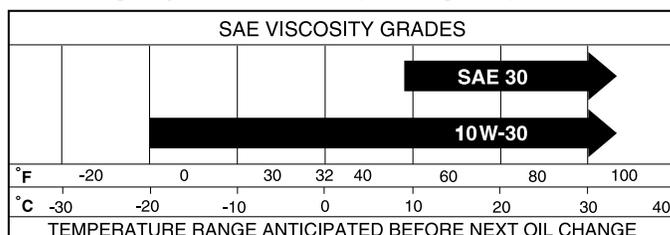
**NOTE:** Multi-viscosity oils (5W30, 10W30 etc.) improve starting in cold weather, and you should check your engine oil level frequently to avoid possible engine damage from running low on oil.
