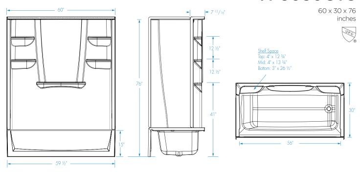
FEATURES Dimensional Tolerance ± 3/8". Dimensions needed for site preparation should be measured from the unit. Manufacturer assumes no responsibility for preparatory work.
