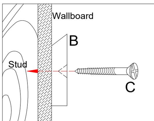
**Step 4:** If hole locations do not align with stud in wall, install the EZ Anchor(D) in to drywall by tapping it in to the predrilled pilot holes up to the thread, and then screwing the EZ Anchor in to the drywall. Attach Cleat (B) using wood screw (C) to EZ Anchors. **NOTE:** Cleat could be secured using combination of Studs and EZ Anchors.
