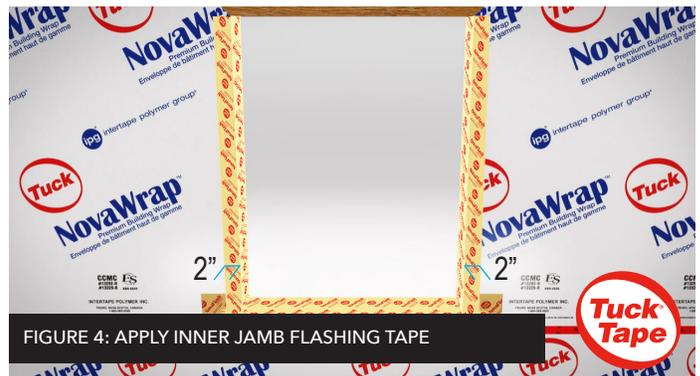
FIGURE 4: APPLY INNER JAMB FLASHING TAPE
