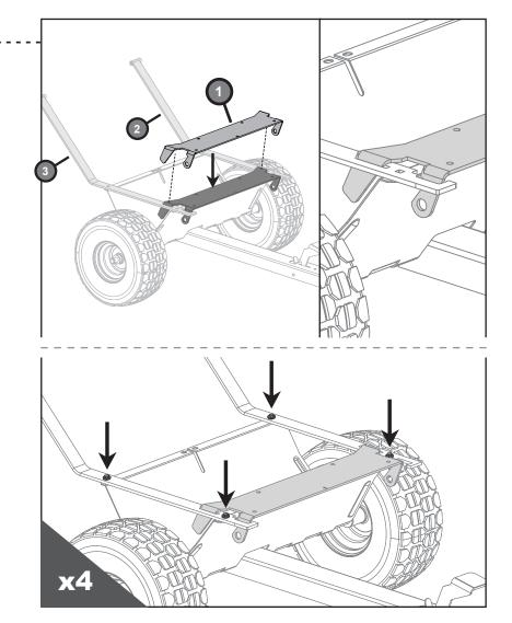
Tighten the four 5/16" nuts (18) from Steps 5-A and 5-B (reference pages 8-9).
