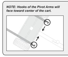
Add both carriage bolts (18) to the Pivot Arm (2) and A-Frame as illustrated here.
