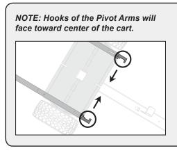
Add both carriage bolts (18) to the Pivot Arm (3) and A-Frame as illustrated here.
