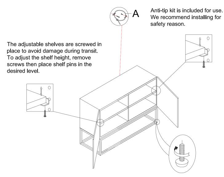
Adjust leveler if needed to level door chest on uneven floor.
