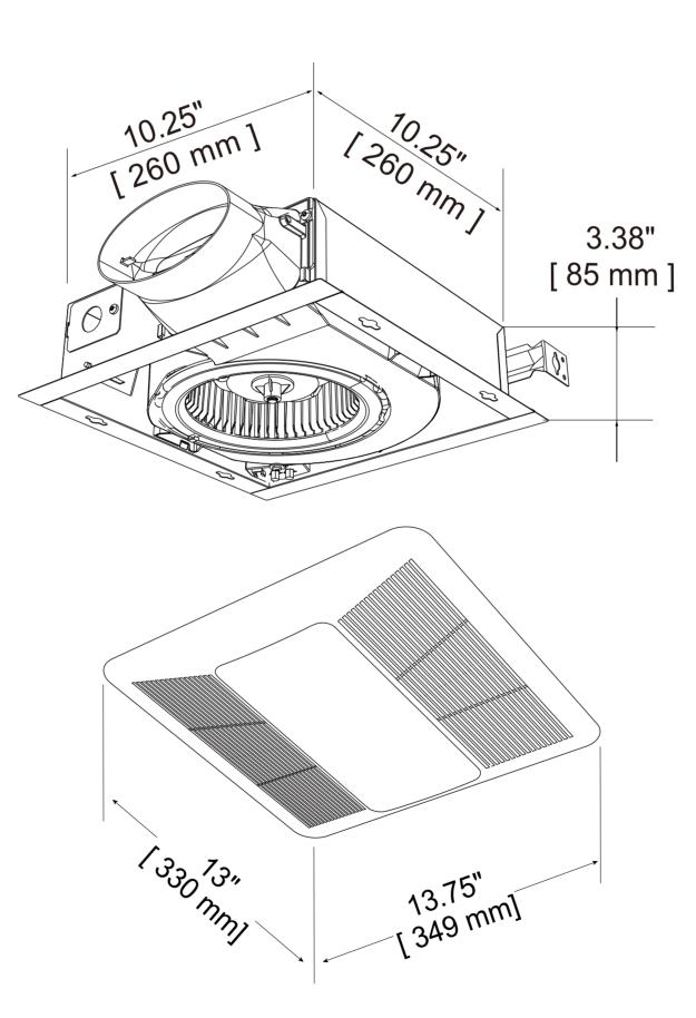
This fan can be installed to 10.5" - 21" between the joist or to I-joists, standard joists and truss construction.
