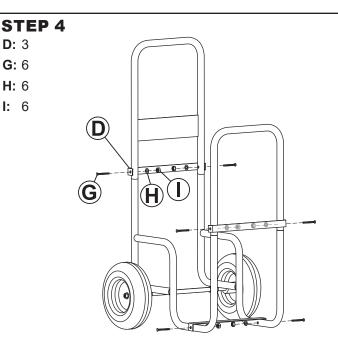
Loosely secure one Brace (D) to the bottom of the log cart by hand-tightening two M8x40mm Bolts (G), two M8 Washers (H) and two M8 Lock Nuts (I).
