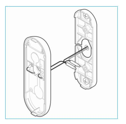
Install the doorbell backplate to the mounting bracket using the included machine screws.
