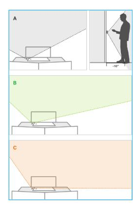
At the installation location, an angled mounting bracket can be used to modify the field of view. Choose a mounting bracket type best suited for your installation setup. Installation scenarios corresponding to mounting bracket types A, B, and C are provided below to guide your decision.
