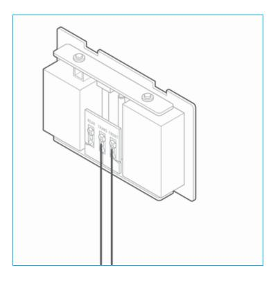
Loosen the screws on the chime associated with the transformer and doorbell. Set the wires aside. Take the power module and hook the curved white wires onto the screw terminals. Tighten the screws. Using a crimp tool and the connectors provided, connect the wires you set aside to the straight grey wires of the power module (either grey wire can be connected to either existing wire). Adhere the power module to the side of the chime. Replace the chime cover.
