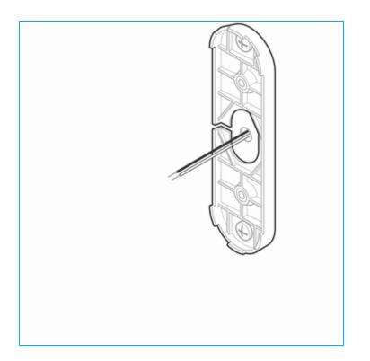
Crimp the two wires coming through the backplate to the existing wires threaded through the mounting bracket.
