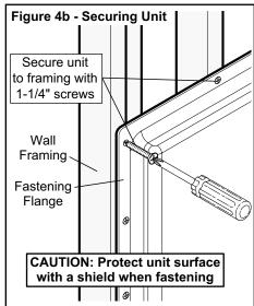
After the unit is confirmed level and square in the alcove, drill a 1/8 inch hole through the fastening flange at each framing member and every 8 inches along the front fastening flanges. Secure the unit in place across the back wall first, followed by the flanges at each end and along the front flanges, using 1-1/4 inch screws or other appropriate fasteners. Continuously check to confirm the unit remains square within the alcove as it is being secured. (Figures 4a & 4b)
