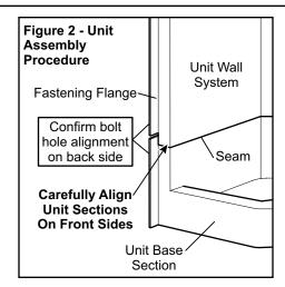
With the wall system in place, adjust one front corner until flush with the shower base front and along the inside surface. Hold the wall in position, while checking the alignment of the hole nearest the corner. If not exactly aligned, carefully
