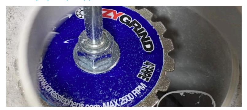
Jones Stephens' Ezy Grind Pipe Cutter cuts plastic DWV and HDPE pipe from the interior of the pipe. The cutter is made from tool steel, is suitable for portable power drills, and has a 1/4" hex shank that fits all drill chucks. The Ezy Grind features a guided cutting motion that allows a pre-set depth of cut.
