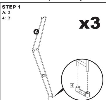
Firmly push one Plastic Foot (4) onto the bottom of Leg (A).
