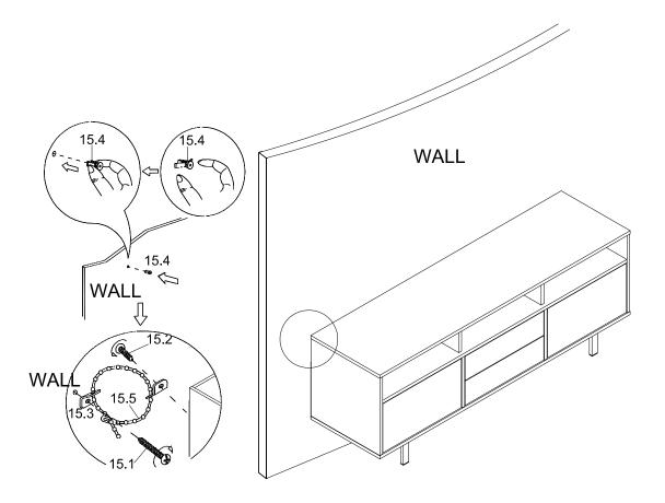
Follow the instructions printed on the plastic bag containing the tipping restraint hardware to attach thetip-over restraints to the unit and the wall.
