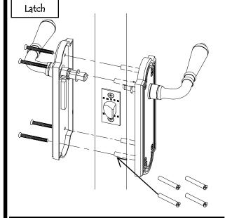
Thru bolts (provided) may be used on hollow doors instead of wood screws (also provided).
