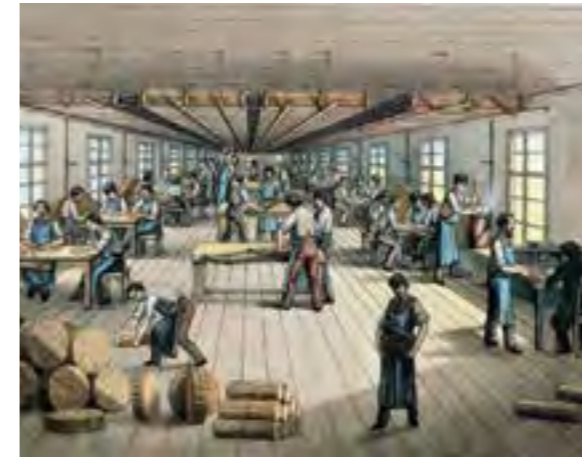
Gluing the graphite into the wooden slats
