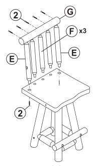
Place two Outer Back Rails (E) into the outside holes on the back of the seat and three Inner Back Rails (F) into the middle holes in the back of the seat.
