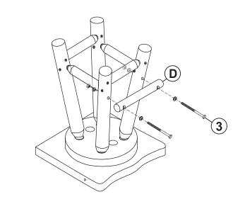
Fasten Footrest (D) to the front legs using two M7x100mm Bolt Sets (3).
