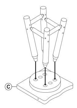
Insert the legs into the underside of Seat (C).
