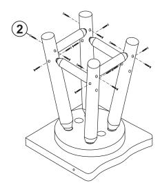
Ensuring the stretcher is fully inserted into the leg, secure each leg to the stretcher using four M3x35mm Screws (2).
