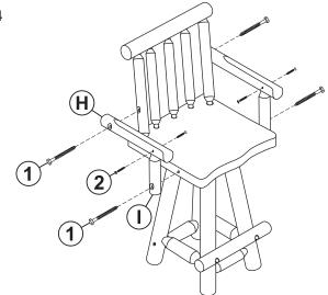
Attach Armrest (H) to the back rail using one M7x80mm Screw (1).
