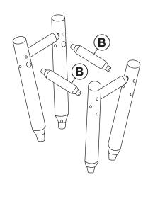
Firmly insert the remaining two Stretchers (B) between the front and back leg sets, as shown.
