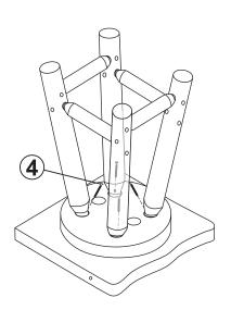
Ensuring the legs are fully inserted into the seat, secure the legs to the seat using four M3x60mm Screws (4).
