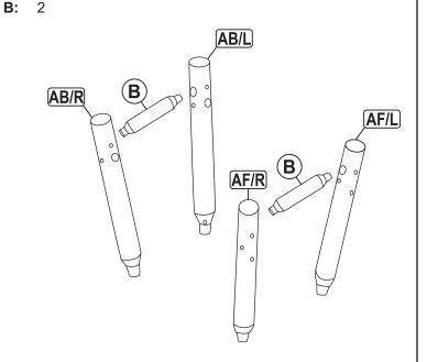
Firmly insert two Stretchers (B) between Front Legs (AF) and Back Legs (AB), as shown.
