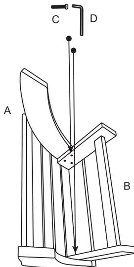
Use 3 Bolts (C) on each side to attach Leg (B) to Footrest Panel (A) with Allen Wrench (D).
