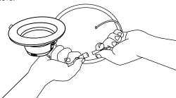
If using an incadescent housing, screw the edison base socket string into the socket. Mate the downlight connector into the Edison (or GU24) base connector.
