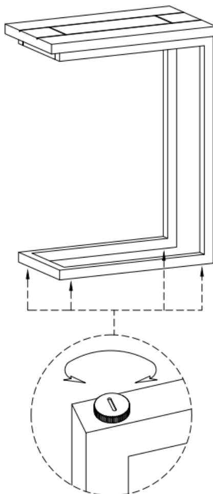
**NOTE:** Levelers on the bottom of the base can be adjusted if floor is uneven.
