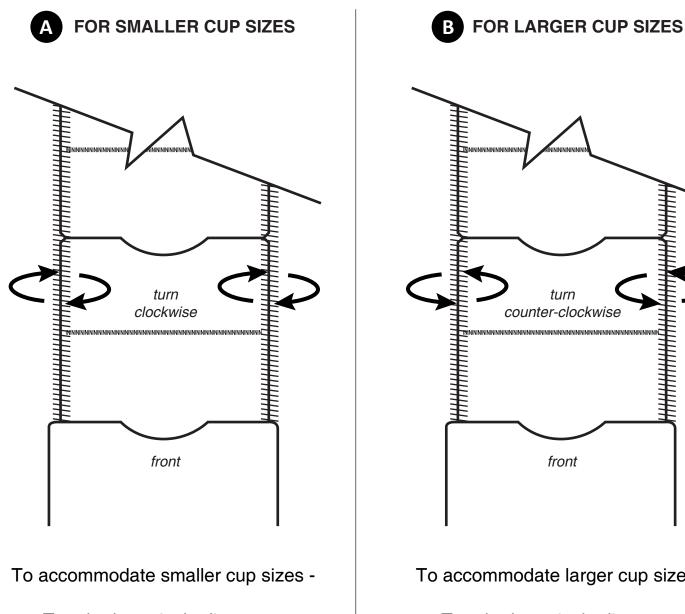
Turn both vertical adjustment springs clockwise at the same time to tighten / shorter tier spacing.
