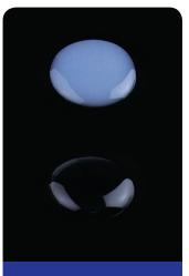
The above tile has 5 coats of floor finish. The top half shows immediate softening of the finish, as indicated by the whitening effect, caused by a high alkaline (11 pH) disinfectant. The bottom half shows that the Virex®II 256 product has no effect, as evidenced by the absence of any whitening.
