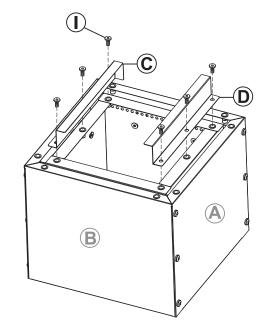
Ensuring the mounting holes face toward the outside of the fire pit, fasten Right Ash Tray Rail (C) and Left Ash Tray Rail (D) to the bottom of the fire pit using six Bolts (I).
