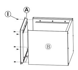
Align remaining Side Panel (A) with Side Panels (B) and loosely secure by hand-tightening six Bolts (I).
