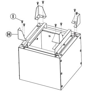
Align four Feet (H) with the corners of the fire pit. Secure each foot with two Bolts (I).
