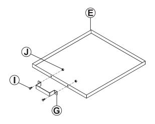
Firmly secure one Handle (G) to Ash Try (E) using two Bolts (I) and two Nuts (J).
