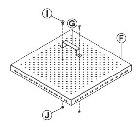
Firmly secure one Handle (G) to Wood Grate (F) using two Bolts (I) and two Nuts (J).
