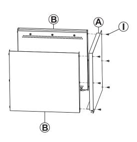
Align two Side Panels (B) with one Side Panel (A) and loosely secure by hand-tightening six Bolts (I).
