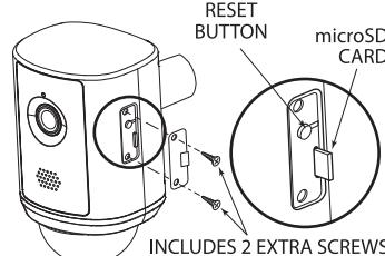
To access Reset Button and microSD™ card, remove cover using a small screwdriver (included). To reset the unit, (unit must be connected to power) press the Reset Button for 15 seconds or until you hear an audible tone. To remove microSD card, push card in with your finger and release. Card will eject halfway.
