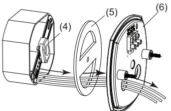
NOTE: Tear away at perforation on Mounting Gasket (5)
