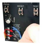
6. Carefully insert the reversed wires into the terminals; you might need to hold the wires in place and tighten the screws at the same time.
