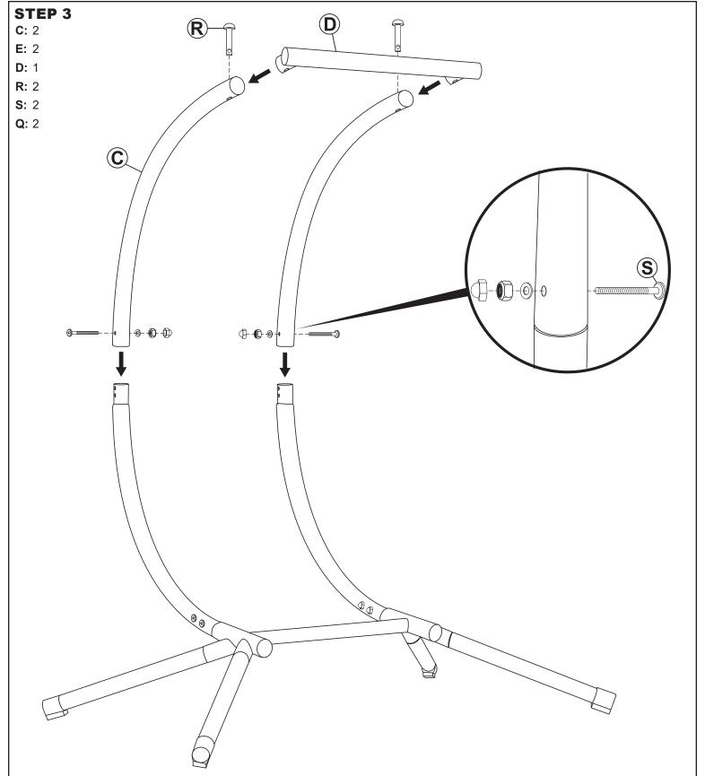
Align each Top Pole (C) with the bottom poles and loosely secure using M10x70mm Bolt Sets (S), as shown. Insert Support Bar (D) into the top poles. Then, place Pin (R) into Top Pole (A).
