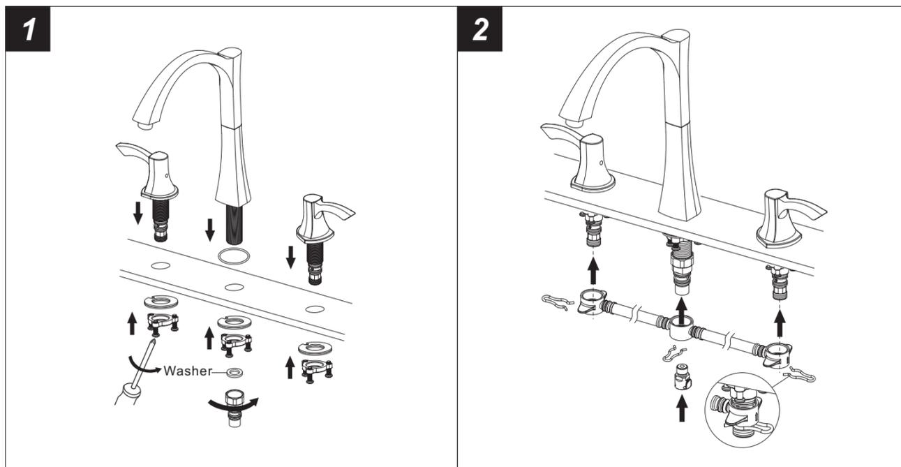
1. Position the faucet and handles on the installation surface and secure them with the fixing kit and tighten the screw with screw driver. Then assemble the diverter assembly. **Warning: don't forget the washer.**
