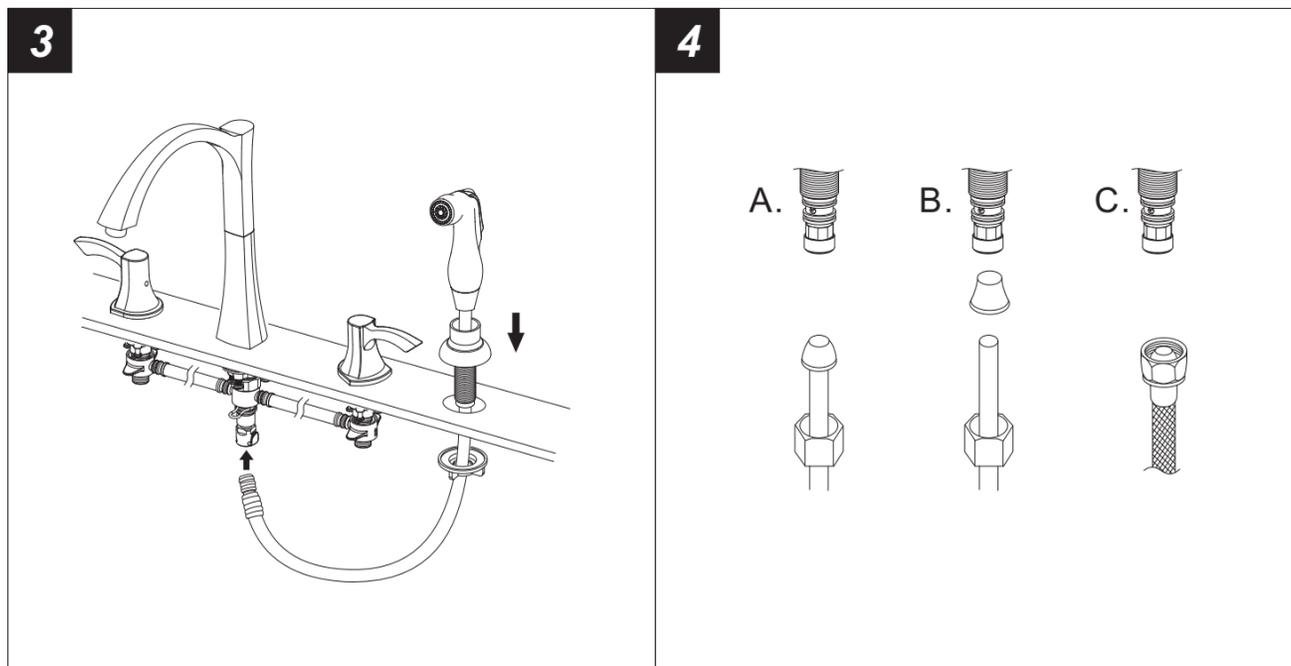
3. Put the side sprayer, base and hose in the installation surface and secure the sprayer with plastic lock nut. And connect the hose to faucet as shown. **CAUTION: Make sure the hose is properly connected to faucet.**
