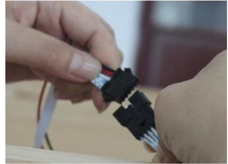
9. Raise the external ROOF COVER above the sauna. Pull the main power cable out through hole in the ROOF and plug securely. Now, secure the ROOF COVER to the sauna with (4) 1-1/8" SCREWS.
