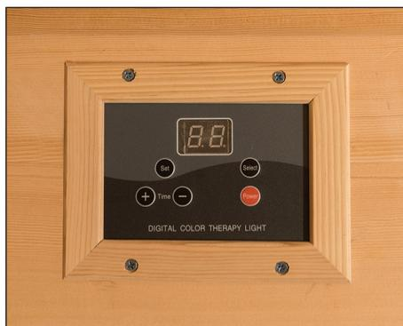
*Note: If you ever need to replace the controller, unscrew from wall and replace faulty controller with new. Plug the 4 and 5 pin wire plugs onto the corresponding connectors on the back, then reattached to wall with screws.*
