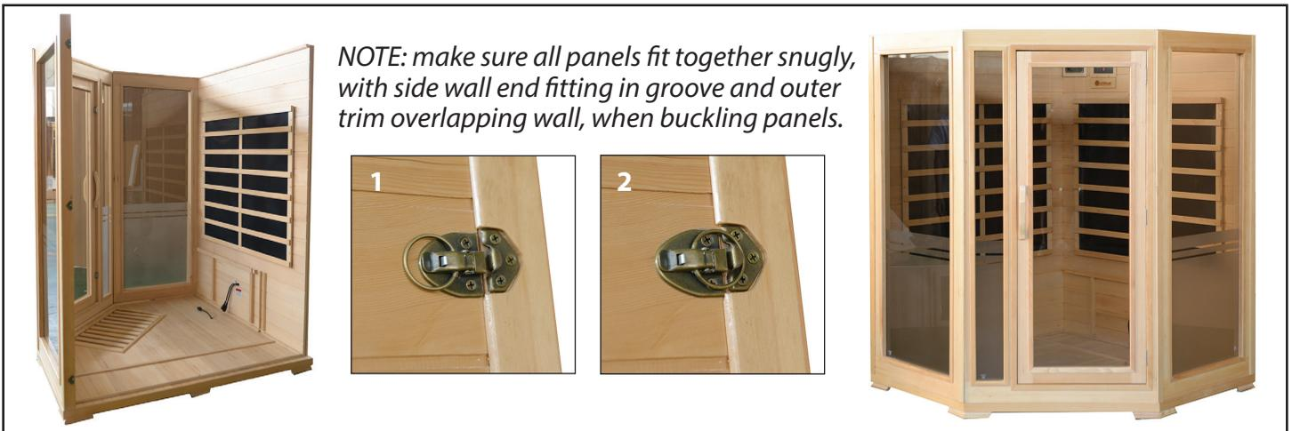
6. Slide the LONG BENCH SUPPORT HEATER PANEL into place between the two SIDE PANELS. Note: It may be necessary to disengage buckles and move a side wall out slightly to do this. Do the same with SHORT BENCH SUPPORT HEATER PANEL, then insert FRONT SMALL BENCH SUPPORTS on either side and attach with (2 ea.) 2" SCREWS.
