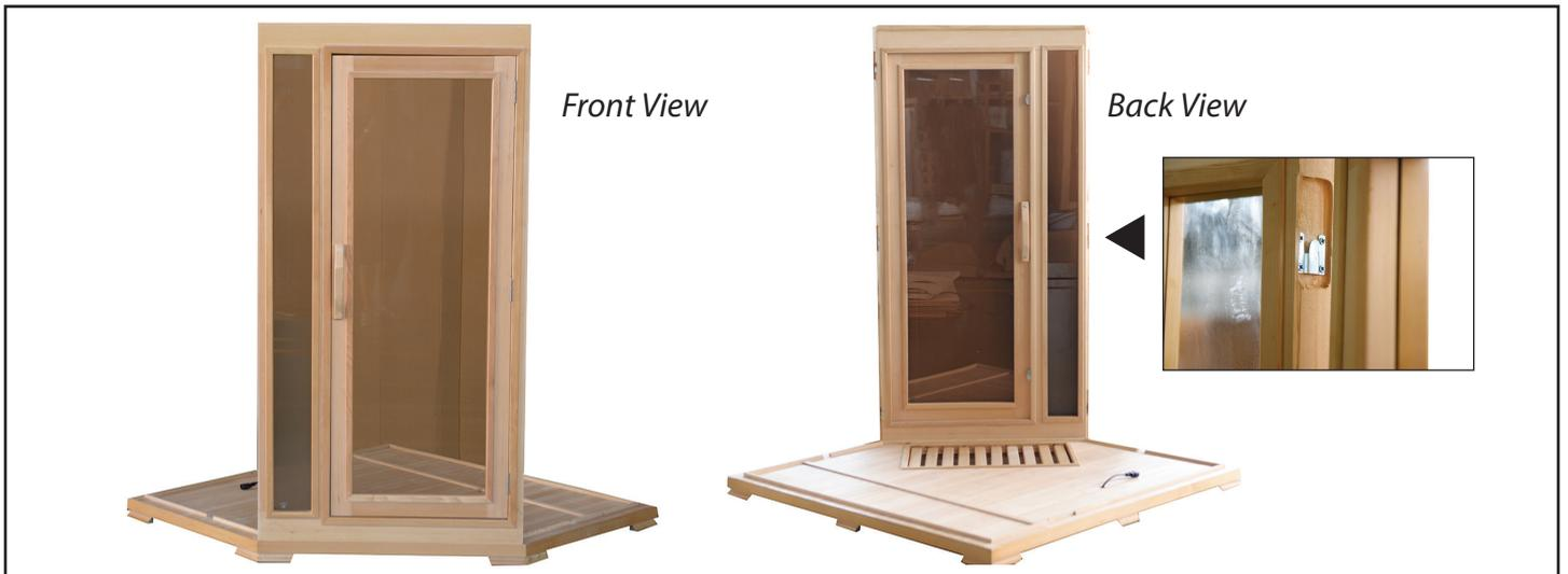
3. Attach the FRONT DOOR PANEL in place by sliding the RIGHT FRONT PANEL down to engage three metal clips on side of door with three brackets on side of RIGHT FRONT PANEL then push down to connect.
