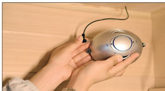
*Note: Press ION to release negatively charged ions to purify the air & press O3 to disinfect the air with ozone.*
