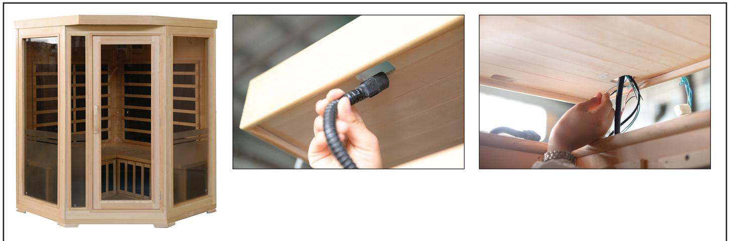
9. Secure the ROOF to the sauna with (5) 1-1/8" SCREWS. Connect the control panel wire, speakers, MP3 player, and heater plugs on the roof to the corresponding wire connections coming up from walls through roof holes.
