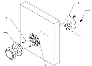
Carefully follow these instructions when installing. Screws to be tightened to a recommended 2.5Nm torque. NOTE:
