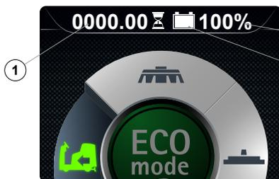
The control display is in the control panel, at the top in the middle it is possible to observe the total time the machine has been used.
