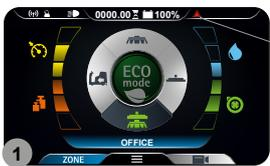
When an error occurs the symbol (1) is displayed in the information field (Fig. 1), it remains visible until the error is resolved. The "ERROR" window will also be displayed in superimposition (Fig. 2), in it are described the number of the alarm, the group it belongs to and a brief description. When an error occurs, do as follows:
