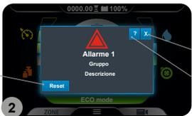
**N.B.:** to close the error screen press the button (3) (Fig.2).
