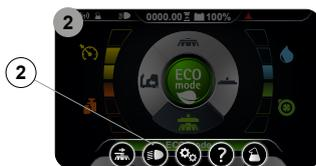
**i** **N.B.:** if the symbol (2) is grey the working lights are not active, if the symbol (2) is green the working lights are active.
