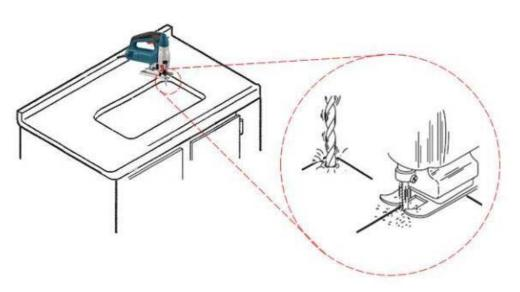
3. Depending on the material used for the countertop it might be necessary to add a support structure made of 2" x 4" or larger lumber around the perimeter of the sink.
