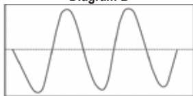
Pure sine waveform typical of home AC outlet
