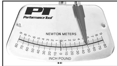
4. The torque scale is calibrated in both Newton Meters and Inch Pounds. Read the applied torque while looking directly down at the pointer, this provides the most accurate reading. Torque can be applied with either a right or left hand pull. The calibration scale has been arranged to aid in reading the numbers regardless of the direction of pull.
