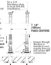
Locate stop valve onto NPT connector with slotted operating screw facing the rear of the installation, fully tighten bottom nut. Check that slotted operating screw has remained in position.
