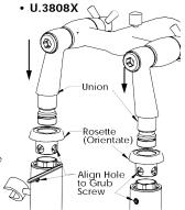
Thread Flex through Rosette onto Bath Union taking care to maintain orientation without twisting the Supply Flex.
