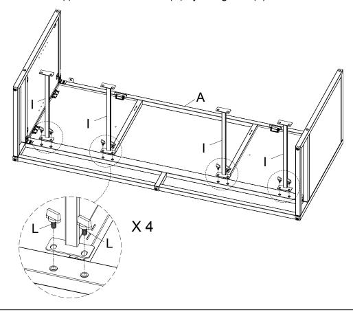
Attach the Back Frame (B) to the Front Frame (A) and Cross Bar (I) by using Bolts (L) as shown.
