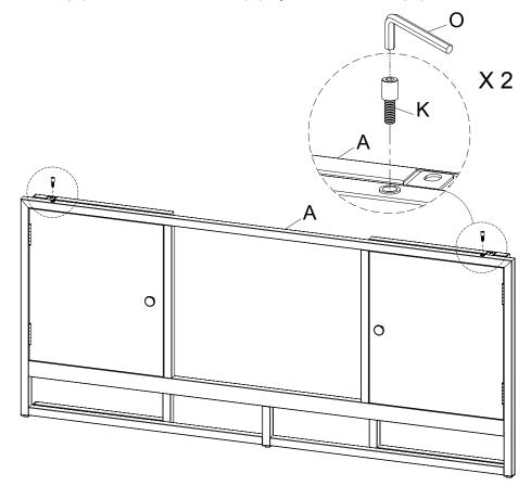
Attach the Bolt (K) to the Back Frame (B) by Allen Wrench (O) as shown.
