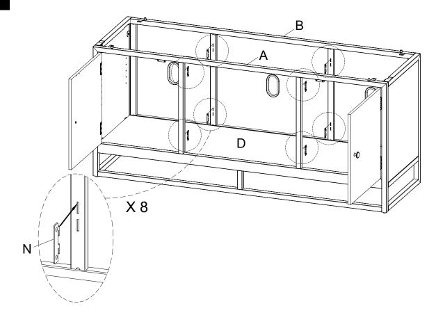
Slide the Divider Panel (E) through the Metal Plate (N). Make sure the dividers are facing correctly as shown.
