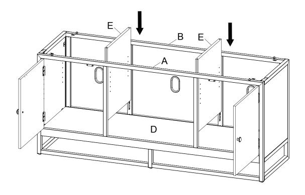
10 Attach Top Panel (C) to the Front Frame (A) and Back Frame (B) by using Bolts (L) as shown.
