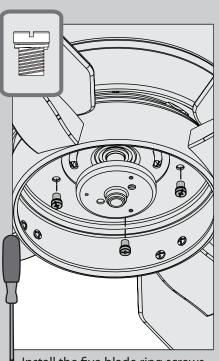
Install the five blade ring screws, found in the X hardware bag.
