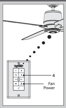
The fan must be paired before it will operate. Press the "4" button and the fan power button simultaneously for at least three seconds. The fan will turn at the lowest speed signifying that the remote pairing process is complete.
