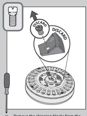
Remove the shipping blocks from the motor. Discard the screws.
