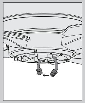
Connect the 9-pin plug connector from the switch housing to the 9-pin plug connector coming from the motor housing. Make sure to line up the colored markings on the connectors.
