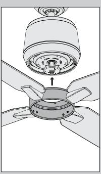
Once all blades have been assembled, lift the blade assembly and align the five screw holes in the blade ring with the screw holes in the motor. It does not matter which set of motor screw holes you choose.
