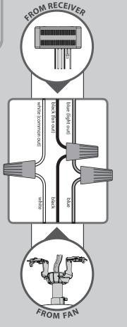
Using an orange wire connector from the hardware bag, connect the black wire (ungrounded) from the ceiling to the black wire from the receiver (marked "live in"). Connect the white wire (grounded) from the ceiling to the white wire from the receiver (marked "neutral in" or "common in").
