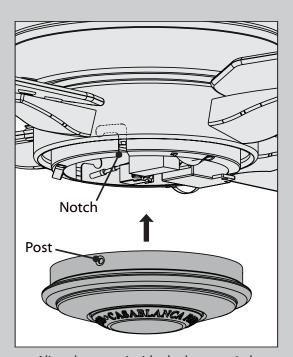
Align the posts inside the lower switch housing with the notches in the upper switch housing. Lift the lower switch housing up as far as it will go, then rotate it clockwise until the posts are held tightly in place by the notches.
