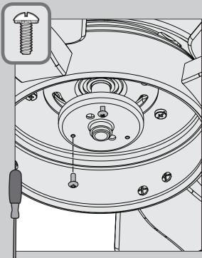
Screw two switch housing assembly screws, found in the hardware bag, halfway into the motor housing. It does not matter which two screw holes you choose.
