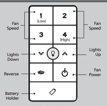
Quickly press the up or down arrow to turn the lights off and on. Hold the up or down arrow to dim or raise the light level. The reverse button changes the direction that the blades turn. The power button turns the fan off and on.
