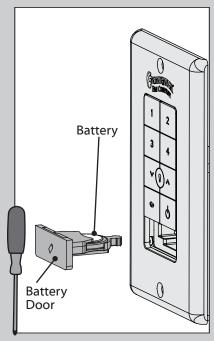
To change the battery, push on the battery door to eject it. Remove the battery using a small Phillip's head screwdriver. Replace with same type battery, making sure the (+) side is facing down. Replace battery holder and battery door.
