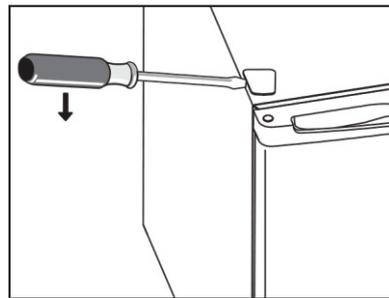
5. Move the core cover from left side to right side. And then lift the door and place it on a padded surface to prevent it from scratching.
