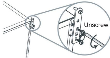
7. Unscrew and remove the bottom hinge pin, turn the bracket over and replace it.
