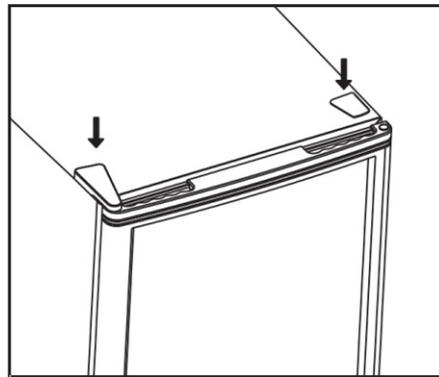
13. With the door closed, check that the door is aligned horizontally and vertically and that the seals are closed on all sides before finally tightening the bottom hinge. Re-adjust the leveling feet as needed.
