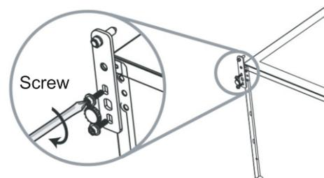
9. Place the door back on. Ensure the door is aligned horizontally and vertically so that the seals are closed on all sides before finally tightening the top hinge.
