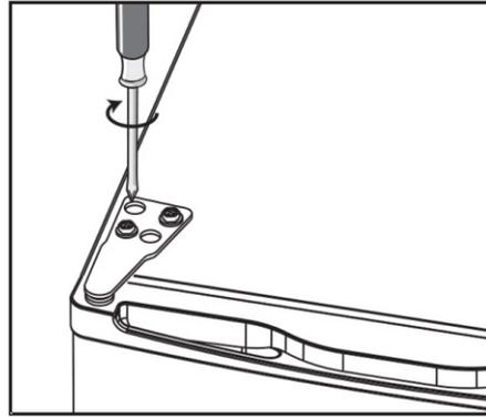
12. Put the hinge cover and the screw cover back.
