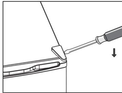
3. Undo the screws. Then remove the hinge bracket.
