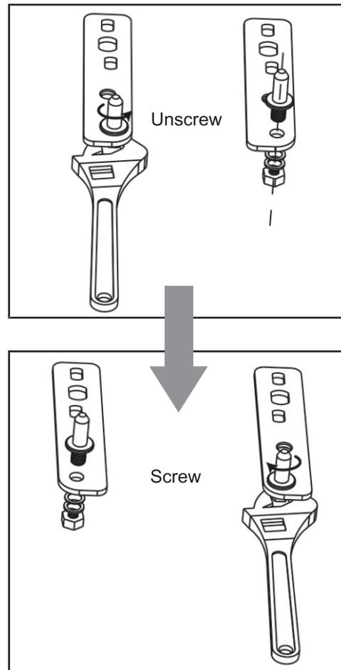
8. Refit the bracket fitting the bottom hinge pin. Replace both leveling feet.
