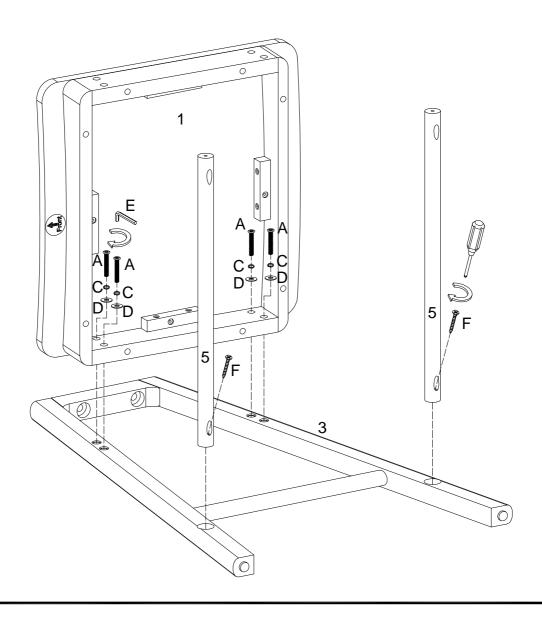
Now, repeat the process for the other side. Secure the Stool Seat (1) to the Right Leg Frame (4) using the Bolt (A), Lock washer (C), and Washer (D). Tighten with the Hex key (E). Next, attach the Support Rails (5) using the (F) Screw. Tighten with a screwdriver.
