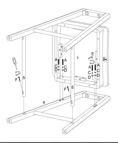
Attach the Stool Seat Back (2) to the chair using the Washer (D), Lock washer (C), and Bolt (B). Tighten with the Hex key (E).
