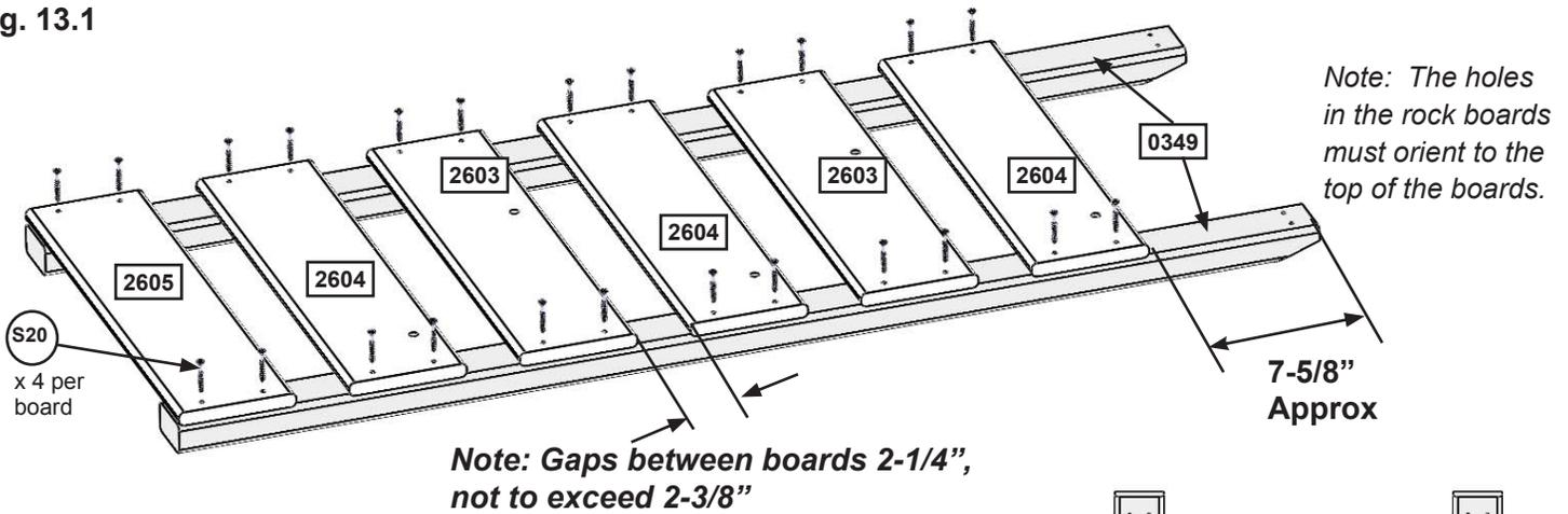
Note: The holes in the rock boards must orient to the top of the boards.
