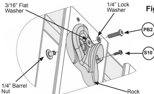
**E:** Place 1 rock on each (2603) Rock Board A and (2604) Rock Board B (fig. 13.2) and attach using 1 (PB2) 1/4 x 1-1/4" Pan Bolt (with lock washer, flat washer and barrel nut) and 1 (S10) #8 x 1" Pan Screw per rock. The Screw must be in the hole directly under the Pan Bolt, it will stop the rock from spinning. (fig. 13.3)
