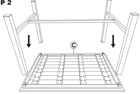
Lay Tabletop (C) facedown on a soft, clean surface.
