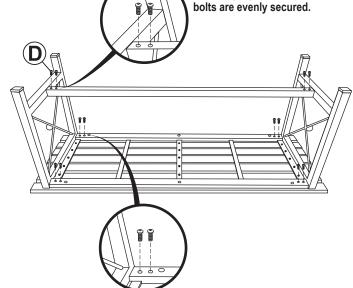
Align the tabs on the top of one Leg Panel (A) with the mounting holes on the opposite side of the metal frame of the tabletop. Secure the crossbar to the legs using two M8x16mm Bolts (D). Then, secure each leg to the tabletop using two M8x16mm Bolts (D).
