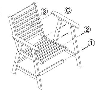
Align Left Arm Panel (C) with the backrest, seat, and stretchers.
