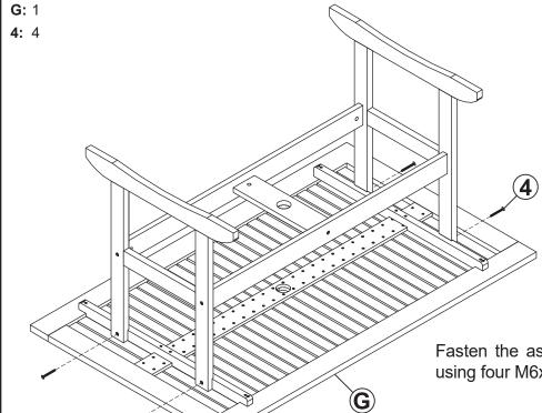
Fasten the assembled table frame to Table Top (G) using four M6x40mm Bolts (4).
