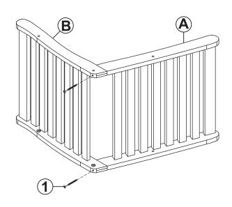
Secure Seat (B) to Backrest (A) using two M6x60mm Screws (1).
