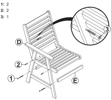
Secure Right Arm Panel (D) to the seat using two M6x30mm Bolts + Cap (2).
