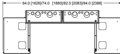
25 [6] MIN. DISTANCE REQUIRED BETWEEN DWR'S USING ZERO CLEARANCE LATCHES
