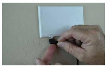
10. Plug the other end of the wire into your tablet. Then, attach the tablet to the S-Mount-P. Route any extra wire behind the tablet so that it is hidden from sight.
