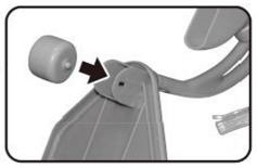
Assemble the front wheel. Apply a little force until the axle of front wheel fits into place.
