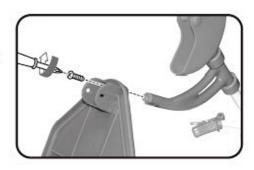
Assemble the small wheel. Just apply a little force to fit the small wheel in place.
