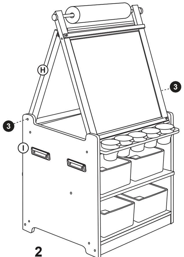
Secure Part H with Hardware 3 on both sides, as shown in above diagram.
