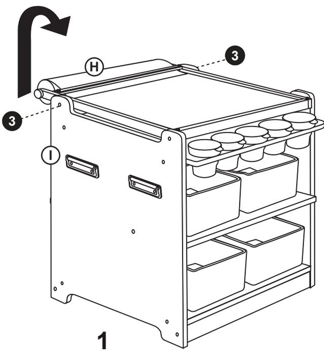
Remove Hardware 3 from both sides of Art Cart. Lift Part H up and allow dowels to rest into the easel position.
