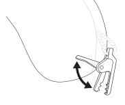
**STEP 7:** To hang the banner, open the clips that are located on the hands of the unit by pulling the lever upward. Place the banner between the teeth of the clip and carefully press the clip lever closed.
