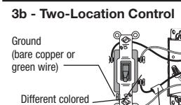
**Two switches controlling a light fixture:**
