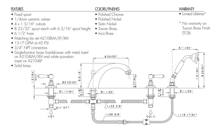
Installation note For servicing after installation, install a service door near the valves
